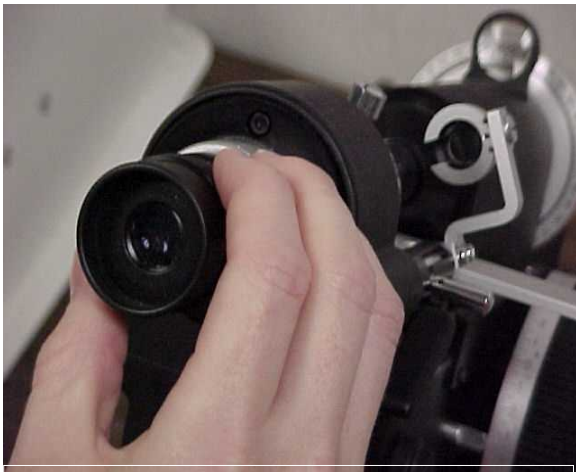
Fig. 1: First focus the eyepiece before
