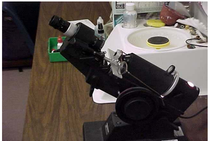
Fig. 2: Place the right lens on stage
