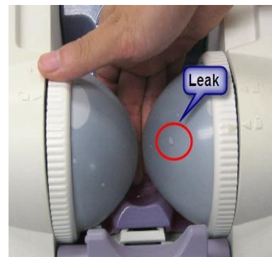
A membrane with a leak
