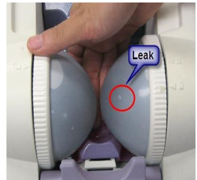
A membrane with a leak
