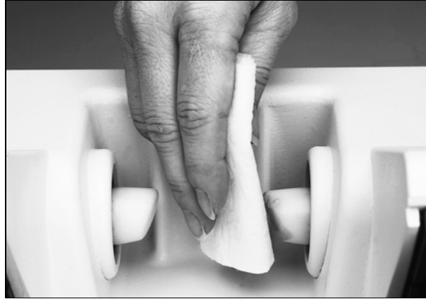
Figure 4-24 Cleaning the Pads
