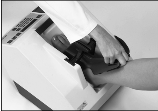
Figure 4-13 Positioning Aid Slightly Loose
