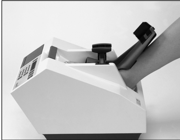
Figure 4-16 Incorrect Leg Angle (system too far)
