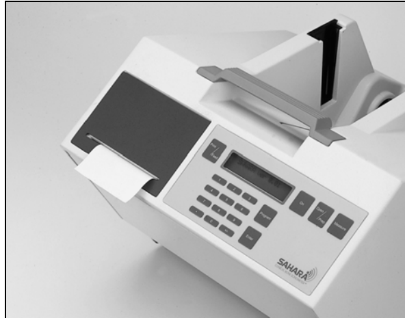
Figure 2-8 Printer Cover Replaced
